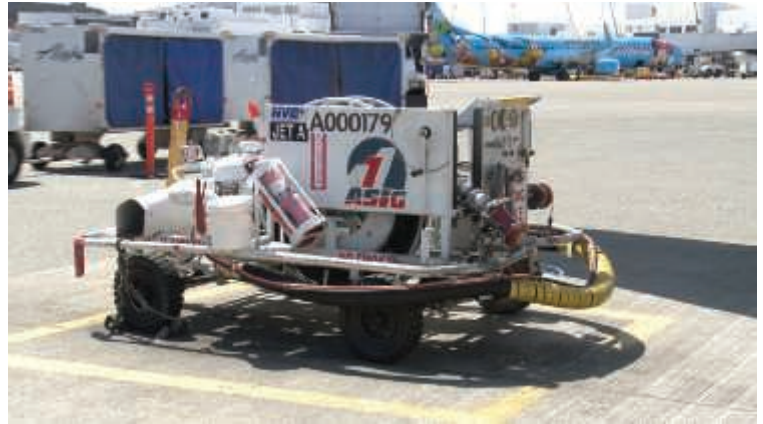
In keeping with 5S, airports, like many other facilities, specify with painted guidelines exactly where tools and equipment such as this fuel pump are to be positioned.
